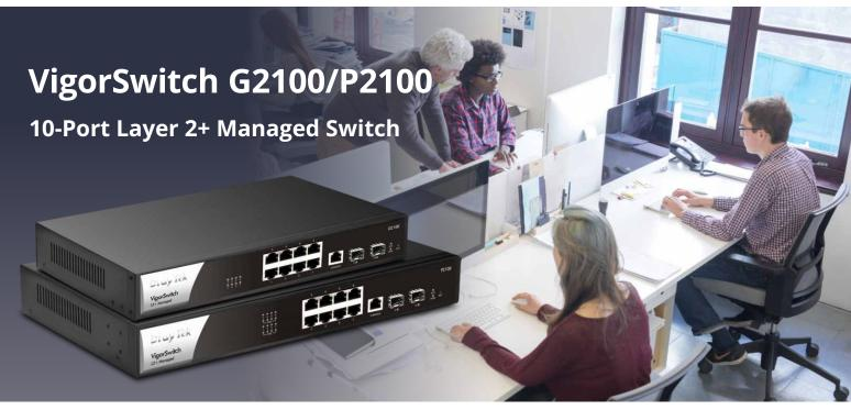
DrayTek VigorSwitch G2100/P2100 is a compact Layer 2+ Managed Gigabit switch well-suited for smart home and branch/remote sites. It has 2x GbE SFP ports, 8x Gigabit Ethernet ports, and 1x console port. Featuring Layer 3 features, including DHCP Server and VLAN Routing. Furthermore with IP Conflict Detection & Prevention, ONVIF Surveillance, ping watchdog and a lot more, this is the balanced switch that brings advanced features into small environments.
