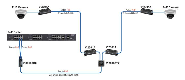
Ethernet and PoE extenders can be used along with the Vi00103 to extend Ethernet and PoE connections. They can be placed on either the switch side or camera side.
