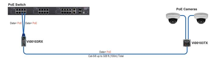
The Vi00103 enables adding an extra PoE camera connection using an existing Cat5/6 cable.
