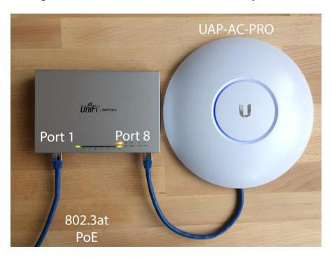
48V Devices CANNOT be powered by 802.3af PoE passthrough:
