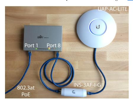
24V Devices CANNOT Be Powered By 802.3af PoE Passthrough with INS-3AF-I-G:
