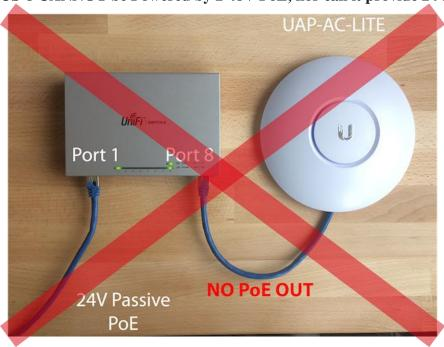
In order to power a 24V passive device on PoE Out, we recommend using a 48V power input, then connecting a 802.3 gigabit adapter (INS-3AF-I-G or INS-3AF-O-G) to PoE Out to convert 48V PoE Out to 24V. Indoor and outdoor 802.3 gigabit adapters are available on the <u>UI Store:</u> Accessories section. As with 48V devices, 802.3af PoE will power the switch, but not connected devices.
