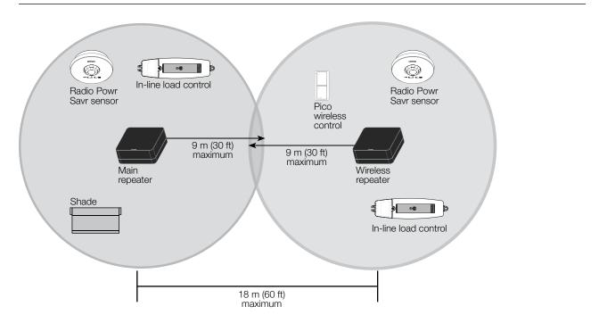
All devices must be located within 9 m (30 ft) of a repeater. The range can be extended with up to four RA2 Select wireless repeaters ( $L\underline{x}$ -REPPRO).
