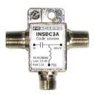
**DC** inserter with F-female connectors. This is used to feed **DC** to the **SWI850X dCSRUK** cascadable system from the top to the bottom; They can also be used to supply **DC** to to the LNBs with the power pass on the inputs and outputs of the multiswitches. (see second installation example).
