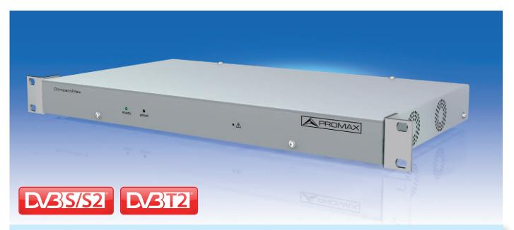
**CompactMax-3** is a compact transmodulation system that allows to distribute Satellite TV channels (DVB-S or DVB-S2) in Second Generation Digital Terrestrial Television (DVB-T2) format. It can be connected to up to **4 satellite inputs** to deliver up to 4 DVB-T2 muxes with dynamic webserver management via remote control. It is integrated into a 19" 1U Rackmount case. It can also be mounted directly on the wall.
