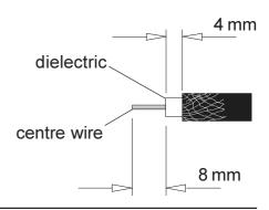
3. Pass the connector over the cable and twist on until the dielectric is flush with the bottom face of the connector. Approximately 2 mm of the centre wire should protrude from the connector (trim if necessary).
