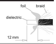
2. Cut away foil flush to the outer sheath. Trim off dielectric as shown to expose the centre copper wire. Ensure that none of the copper braid touches the centre wire.
