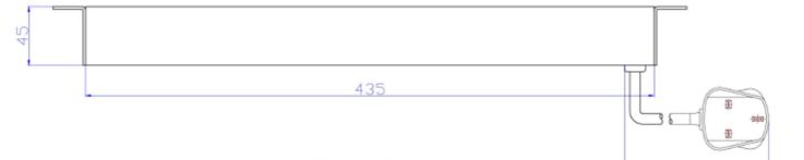
3Gx1.5mm²x2.5m Net length ,UK plug ,cable enter on the back
