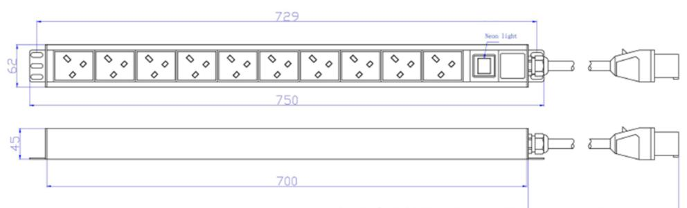
3Gx6mm<sup>2</sup> x2. 5m Net length, 32A commando plug
