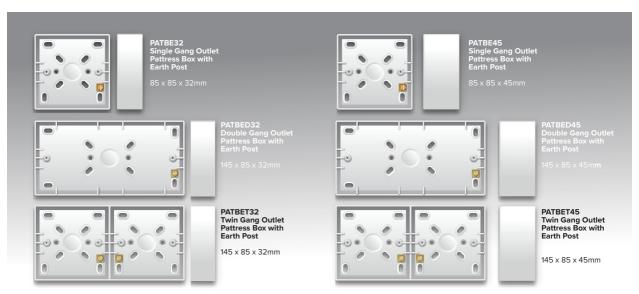
Our range of pattress boxes with additional earth posts are available in 2 depths to suit various installation needs. Made from durable ABS with added strength and a selection of punch out sections for easy installation.
