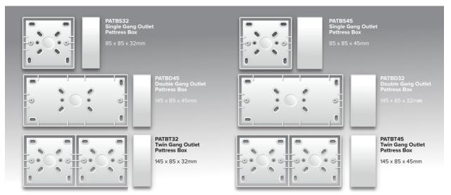
A comprehensive range of pattress boxes available in a number of depths to suit a variety of installations needs. Made from durable ABS provides added strength with a selection of punch out sections for easy installation.
