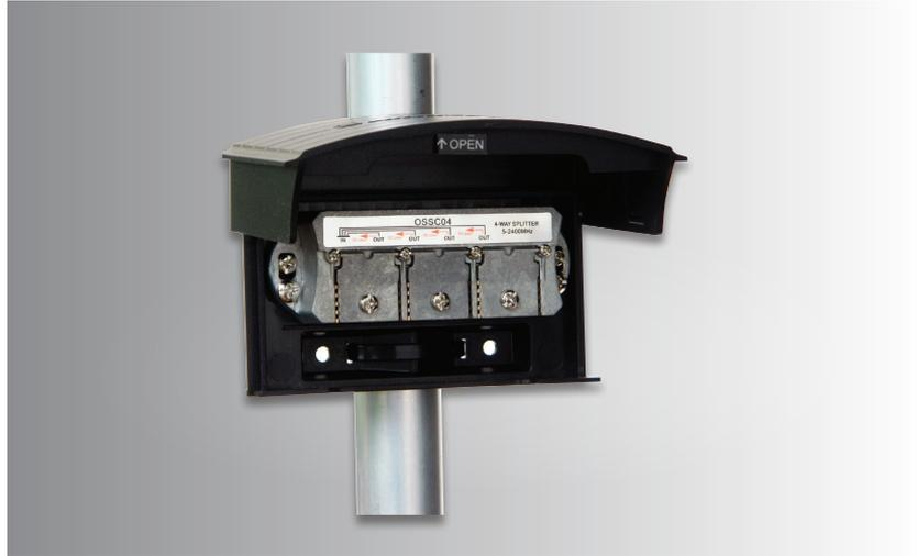
The compact masthead splitters are a neat range of outdoor splitters with a clever hinge design that allows them to be mounted under an eave. They are fully screened with saddle and clamp style connections and a DC pass to allow use with a masthead amp and PSU if required.
