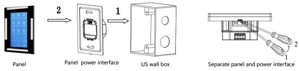
Installation: Hold the edge of the panel (shown as above grey area), insert the power interface module vertically. Do not push the panel too hard.
