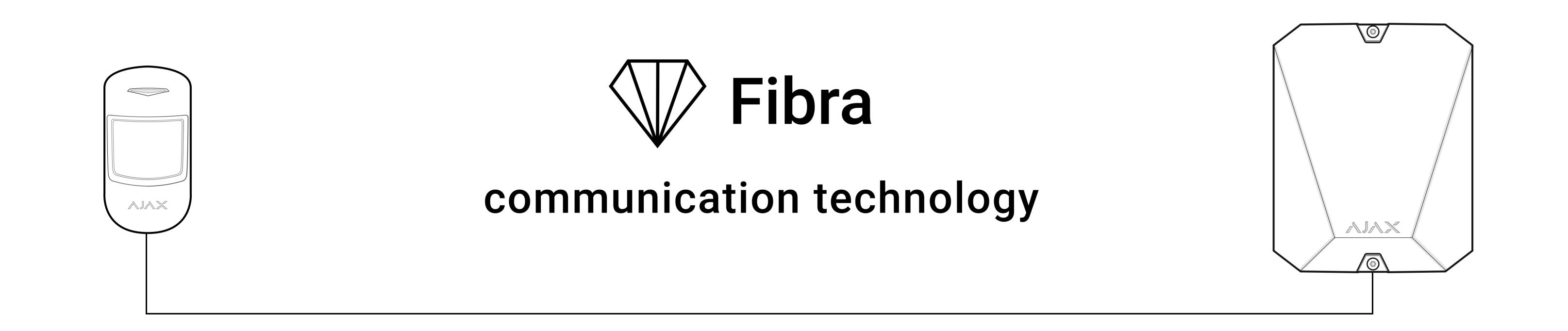
Fibra is a two-way wired protocol, ensuring fast and secure communication between hubs and devices. Based on a **bus connection method**, Fibra delivers instant data-rich alarms: security companies and users know which device was triggered, when and where it happened.
