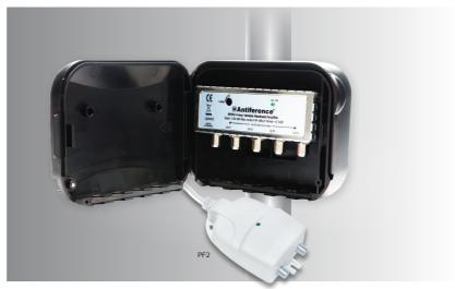
Fully screened masthead amplifier kits with variable gain & F connections to boost television signals to optimum levels. Optional outputs of 1, 2 or 4 gain adjustable from 1-20dB. Weatherproof housing & kits include power supply.
