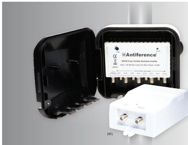
Masthead amplifier kits for larger installations. With variable gain control 1-25dB and fully screened with F connections, distributes television signal to 6 or 8 TV sets. Power supply can be fitted to any of the output locations.
