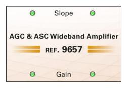
The 2 LEDs on the left indicate the Slope and Gain status of the left SAT input.
