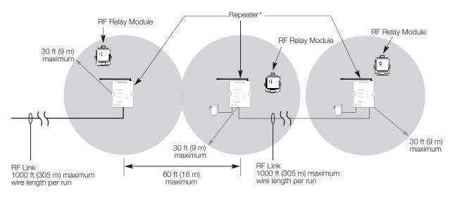
\* In HomeWorks systems, use hybrid repeaters for range extension. In RadioRA 2, the repeater shown may be either a main repeater (1 required) or auxiliary repeater (up to 4 permitted).
