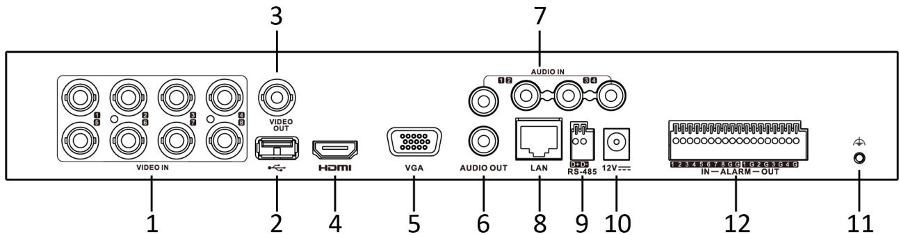
\*: The rear panel of iDS-7204HUHI-K1/4S(B) provides 4 video input interfaces.
