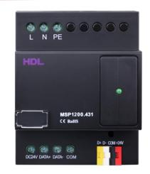
HDL-MSP1200.431 is a power supply module. The module can supply DC24V voltage, 1200mA current. It has 2 kinds of connection types, the total current is 1200mA
