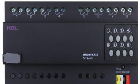
**HDL-MR0810.432** Intelligent Relay Module, has 16A launching relay inside, Zero power consumption and high reliability. The relay's communication interface is HDL Bus Pro, which is based on RS485 protocol.
