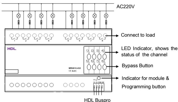
**Indicator for module:** Flickers when the module is working properly. Keep pressing the indicator for 3 seconds, it will turn to red, then user can read and modify the address of the module in the HDL Bus Pro set up software.
