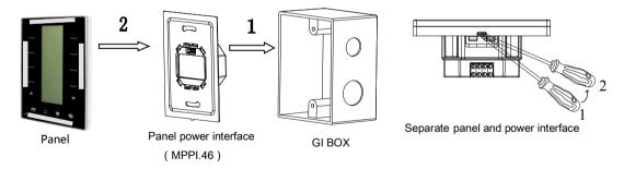
Installation: Held the edge of panel (shown as above grey area), insert the power interface module vertically. Do not push the panel too hard.
