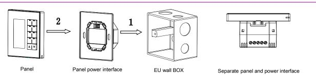
Installation: Hold the edge of panel, insert the power interface module vertically. Do not push the panel too hard. Split: Panel and panel power interface by magnetic suction, you can split them apart directly.
