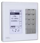
HDL-MPL8-RF.18-A 8-button wireless panel is a new generation of wall-mounted switch with new design. It has 8 control buttons and the left & right side of the button can be programmed separately. 2 buttons are used for the page switching. Each button can be displayed with an icon in the LCD screen, which is customized for final user.
