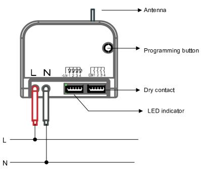
Programming button: if it is working properly, the green light will flicker, press the button three times continuously, the green light will flicker quickly, enter the setup mode (the gateway should enter the setup mode at the same time, and then, set the parameter)
