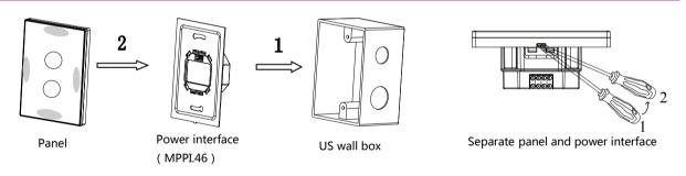
**Installation:** Hold the edge of panel (shown as above), insert the power interface module (MPPI.46) vertically. Do not push the panel too hard.
