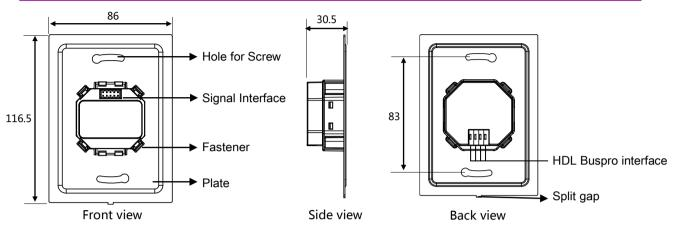
Signal Interface and fastener: To be connected with the panel switch or sensor.
