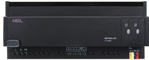
**HDL-MDT0203.433** Dimmer is based on the technology of MOSFET. It has 2 output channels and manual switch is available for each channel. Each channel can choose leading edge or trailing edge by software. This is very useful when user has different type of loads. And it has short circuit protection and over heat protection
