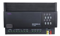
HDL - MDLED0605.432 6 channel 5A Intelligent LED Dimming Module , it can be used to control the LED light which has constant voltage. It has 6 output channel, each channel has a bypass button for manual control. Scene and sequence functions are available.
