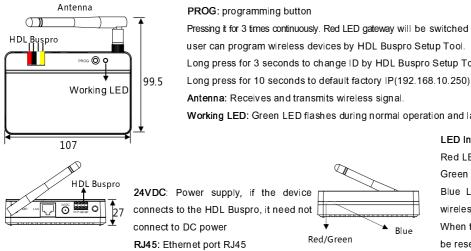
Pressing it for 3 times continuously. Red LED gateway will be switched to set channel for Parameter settings, user can program wireless devices by HDL Buspro Setup Tool
