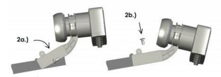
Connect each of the coax cables to the outlets on your new LNB and pull down the weather shield
