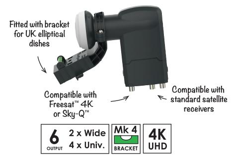
The GH6LB is a Hybrid LNB which means that it combines two different systems for delivering the signal from the satellite to your receivers. The front two outputs are Wideband specifically set-up to be compatible with Freesat™ 4K or Sky-Q™ while the four outputs at the back can feed signals from the same satellite to standard or HD receivers or PVR's.
