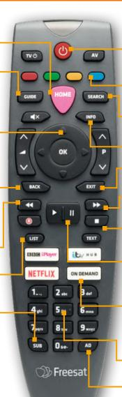
**Power** – turns the Box on and puts it into standby mode
