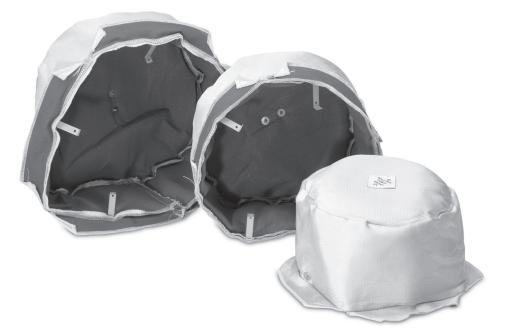
Fire protection and sound absorption when using Q Acoustics and Audica Install speakers can be achieved with the Q Acoustics Install Fire and Acoustic Hood range. Unlike most Fire Hoods available these have been tailor-made to fit all our In-ceiling and In-wall speaker models as listed below. The hoods maintain fire rating integrity of the ceiling to which they are fitted, thus enabling 30 minutes or 60 minutes of fire rating to be maintained.
