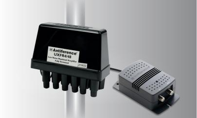
This 4-way masthead amplifier with variable gain control has two inputs UHF and the unique VHF input allowing distribution of FM & DAB signals within the same system. It is fully screened with F-Type connections and housed within a weatherproof case for ultimate weather protection.
