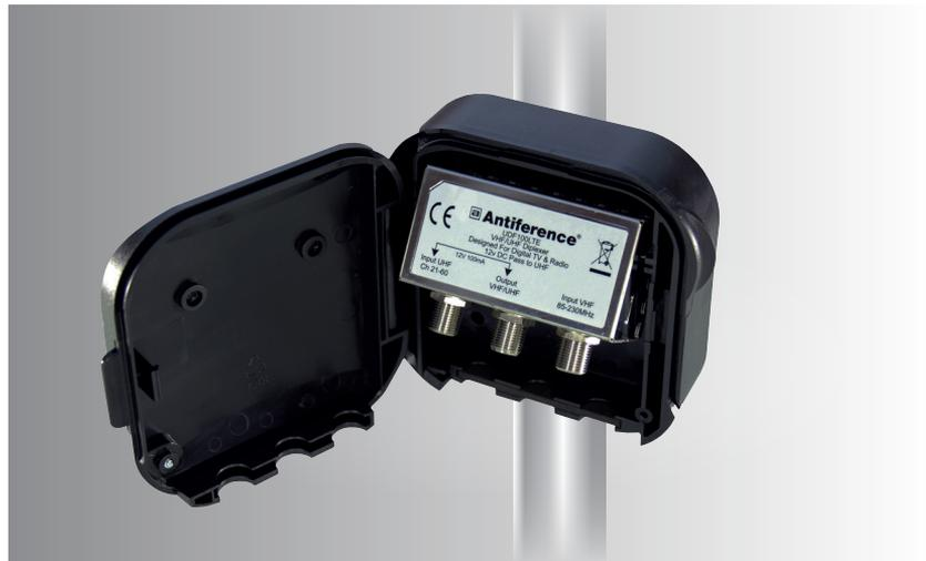
Masthead diplexer for combining UHF & VHF signals onto a single coax cable. 'Tried and tested' weatherproof housing and fully screened with F connections. DC pass on UHF for use with pre-amp.
