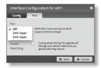
Note: If the PoE screen states that PoE is not supported, then there is insufficient power. You will need to increase the power input to the EdgePoint.
