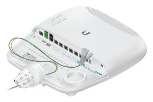
3. Separate the fiber optic strands and spool them around the strain relief reels in the direction of the arrows. Then connect a fiber optic strand to the fiber module.
