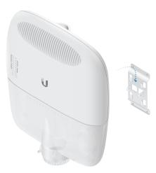
3. Use the two *Phillips Bolts* to attach the EdgePoint to the *Wall-Mount Bracket*.
