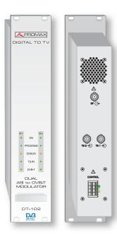
The **DT-101** (single) and **DT-102** (dual) modules are COFDM modulators compatible with DVB-T standard. They have TS-ASI input and RF output in the UHF band and are agile in frequency and output level. Inputs can contain services in all sorts of formats: SD, HD, MPEG-2, MPEG-4, etc.
