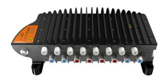
Introducing the new dCSS SwitchBlade from Global Invacom. Featuring 4 x dCSS outputs that support SKY Q and legacy SKY Set top Boxes, 8 x Legacy outputs that support multisatellite up to 4 satellites. SwitchBlade can be used in conjunction with both the ODU32 or Optical LNB. Compatible with existing 8 way SatPlus units. Connector inserts colour coded to aid identification of ports.
