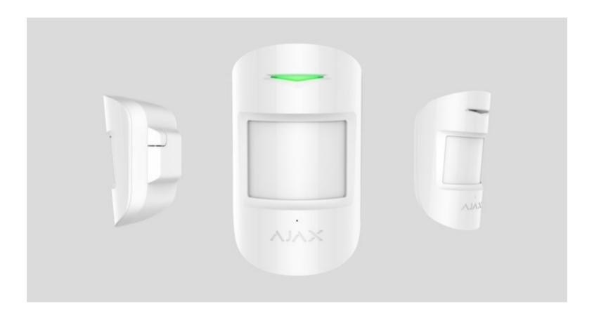
**CombiProtect** is a device combining a wireless motion detector with the viewing angle of 88.5° and distance up to 12 meters, as well as a glass break detector with the distance up to 9 meters. It can ignore animals and detects a person within the protected zone from the first step. It can operate for up to 5 years from a pre-installed battery and is used inside premises.
