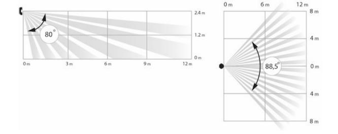
If the detector is not installed at the recommended height, this will reduce the area of the motion detection zone and impair the operation of the function of ignoring animals.
