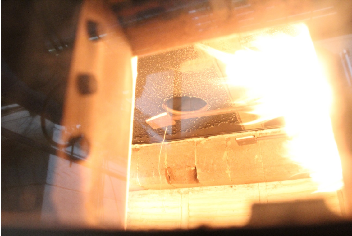
Photo 7 – 5 minutes into test on exposed side, the Hoody fireproof covers are still intact
