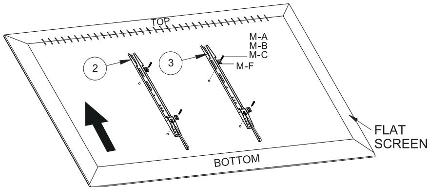
Lay screen flat on the floor (use cloth to prevent scratches to screen). Align interface arms to fixing holes on rear of screen, choose the appropriate size and quantity screws (with multi-washer) according to the mounting holes on screen.
