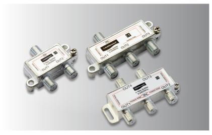
Wideband fully screened F-type splitters for indoor use. Split signals to 2, 3 or 4 TV sets. DC pass feature on all ports is included to allow use of masthead amplifier. Fitted with integral earthing point.
