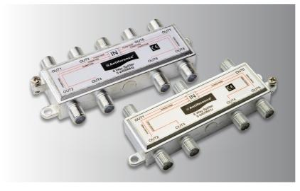
Fully screened wideband F-Type splitters with DC pass on all ports for larger installations. Split signals indoors to 6 or 8 TV sets. Integral earthing point included.
