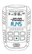
In the test interface of OPM, long press the dB key to display the word "RJ45" on the screen. At this time, enter the RJ45 cable sequence test, connect one end of the network cable to the RJ45 port in the bottom, and connect the other end to the remote tester. Short press the dB key to exit. Long press the dB key again,
