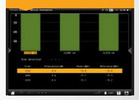
Once the optical fibre input enabled, and thanks to the optical receiver (whether selective or not), optical attenuation measuring can proceed for three wavelengths (1310 nm, 1490 nm, and 1550nm) and their powers, as does RFoG installation analysis.
