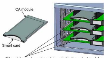
CA modules and smart cards inserted in the output modules
