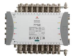
Cascade multiswitch for 1 Satellite position with 5 inputs and 5 trunk outputs, suitable for distributing satellite and terrestrial signals in small to large sized systems. Available with 32 subscriber outputs and powered by the TMS PSU external power supply either directly or via the SAT trunk lines.
