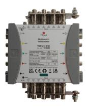
Cascade multiswitch for 1 Satellite position with 5 inputs and 5 trunk outputs, suitable for distributing satellite and terrestrial signals in small to large sized systems. Available with 16 subscriber outputs and powered by the TMS PSU external power supply either directly or via the SAT trunk lines.
