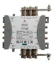
Cascade multiswitch for 1 Satellite position with 5 inputs and 5 trunk outputs, suitable for distributing satellite and terrestrial signals in small to large sized systems. Available with 12 subscriber outputs and powered by the TMS PSU external power supply either directly or via the SAT trunk lines.
