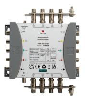
Cascade multiswitch for 1 Satellite position with 5 inputs and 5 trunk outputs, suitable for distributing satellite and terrestrial signals in small to large sized systems. Available with 8 subscriber outputs and powered by the TMS PSU external power supply either directly or via the SAT trunk lines.
