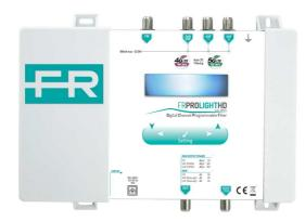
The Fracarro FRPRO LIGHT HD profiler is a flexible and programmable compact high-selectivity headend, equipped with an innovative technology, that allows to filter, convert, amplify and distribute many DVB-T/T2 digital terrestrial multiplexes available in VHF/UHF band with the possibility to mix also the FM signal on the output distribution.
