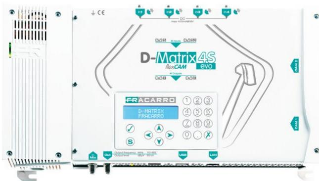
D-Matrix series, compact head end for transmodulation from 4 DVB-S2 trasponders to 4 DVB-T multiplex, 3 flex common interfaces
