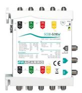
**5-input cascadable SCD2 (dCSS)** multiswitch with CAG; compatible also with **Wideband LNBs; 2 output taps** with 16 frequencies each and **operating mode autodetection**, entirely fed by **DC-IN connector**, **VL line** or by the receivers. SKY Italian frequencies.
